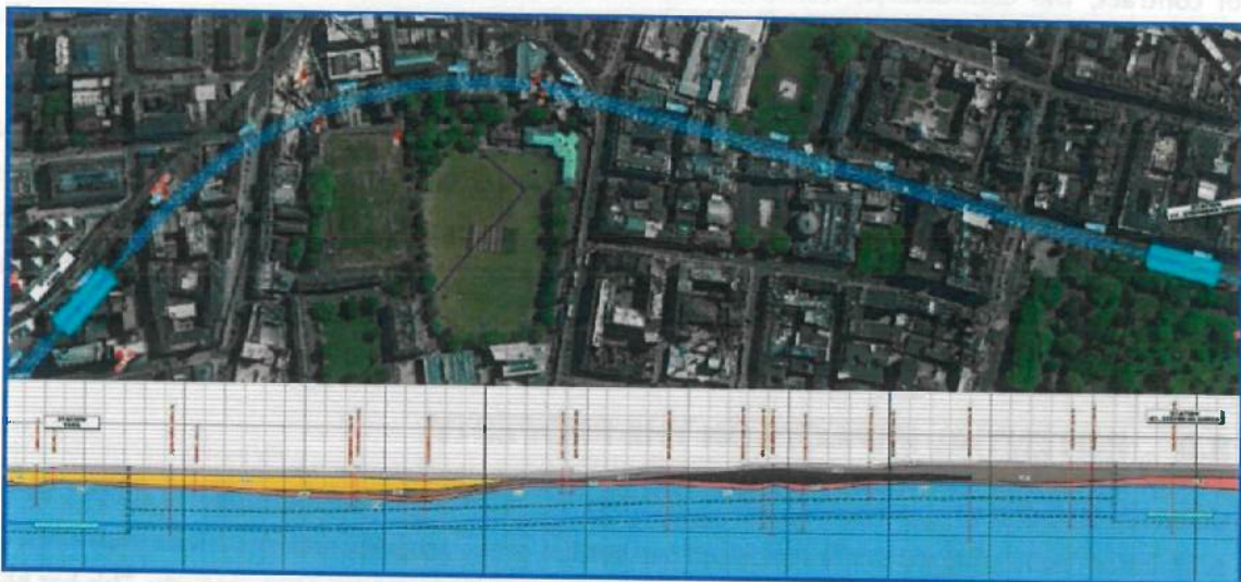
Figure 6. C8 Geological Section (ref. A5.13, Diagram 3.13: Geologic Profile for TBM Drive C8- Tara Station to St. Stephen's Green)
